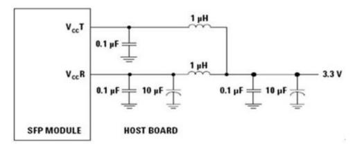
Note: Inductors with DC resistance of less than  $1\Omega$  should be used in order to maintain the required voltage at the SFP input pin with 3.3V supply voltage. When the recommended supply filtering network is used, hot plugging of the SFP transceiver module will result in an inrush current of no more than 30 mA greater than the steady state value
